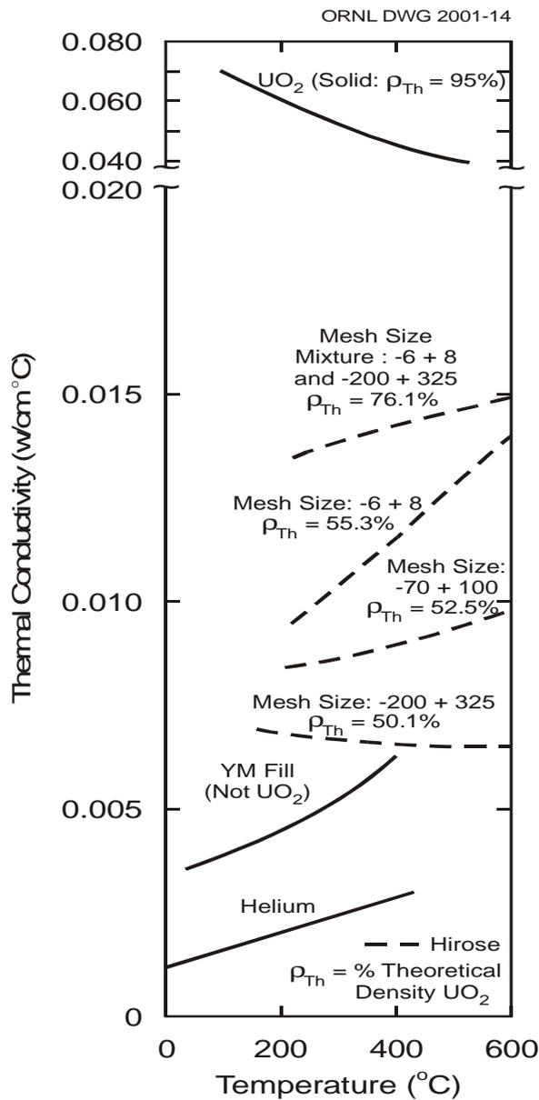
**Fig. 2. Measured thermal conductivity for uranium dioxide particulate beds in helium (1 atm).**
