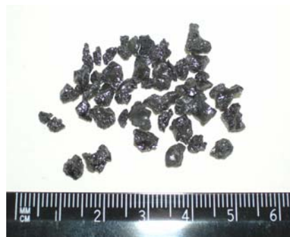
Fig. 7. Particles of melted uranium dioxide with diameter 3-8 mm.
