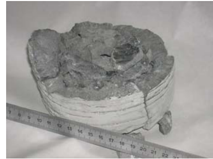
Fig.2. Monolith zirconium dioxide by mass 6 kg.
