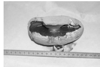
Fig.3. Melted and drained zirconium dioxide
