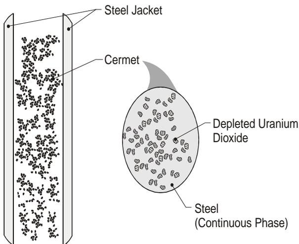
Fig. 1. A Cermet is a CERamic METallic Composite
