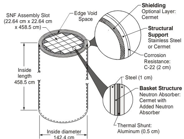
Fig. 3. Uses of Cermet in PWR Spent Nuclear Fuel WPs.
