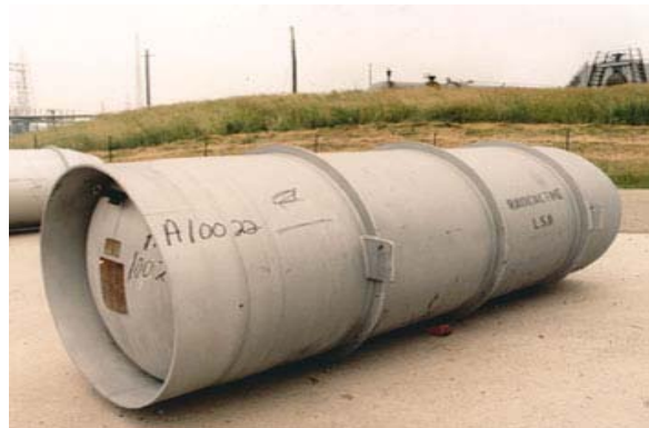
FIGURE 1.1 Typical 12-metric-ton Depleted \text{UF}_6 Storage Cylinder
